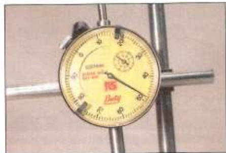
3.17 Dial gauge reading of 1.48 mm
