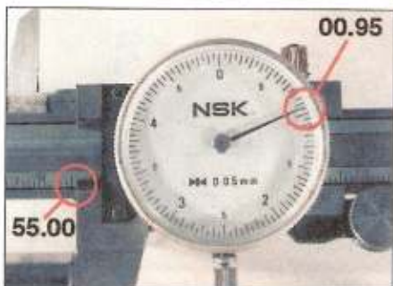
3.14 Vernier gauge reading of 55.95 mm
