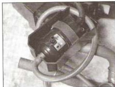
7.7 To renew the separator, disconnect its hoses and remove it from the bracket
