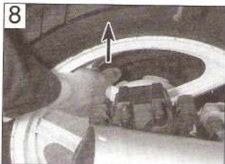
Checking for rear suspension linkage play
