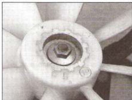
4.7 The fan blade assembly is retained to the motor shaft by a single nut
