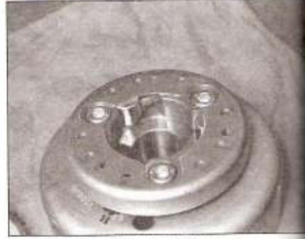
35.10b . . . then install the rollers and release the springs
