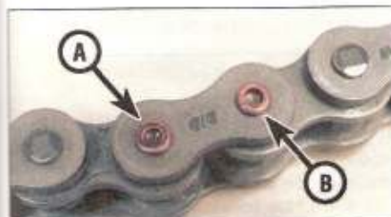
8.9 Pin end correctly riveted (A), pin end unriveted (B)
