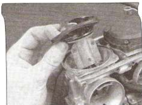
7.4 Remove the diaphragm/piston assembly from the carburettor body
