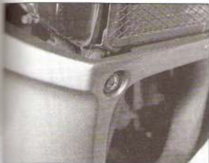
2.2a Lower fairing is secured by two bolts with washers at the front ...
