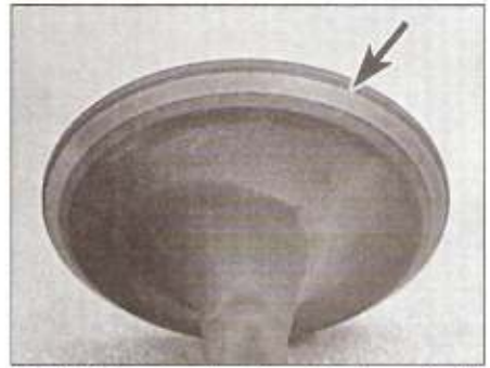
12.24b After lapping, the valve face should exhibit a uniform, unbroken contact pattern (arrowed) . . .
