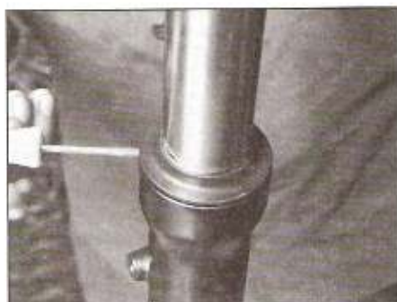
7.6 Pry the dust seal out of the outer tube with a small screwdriver
