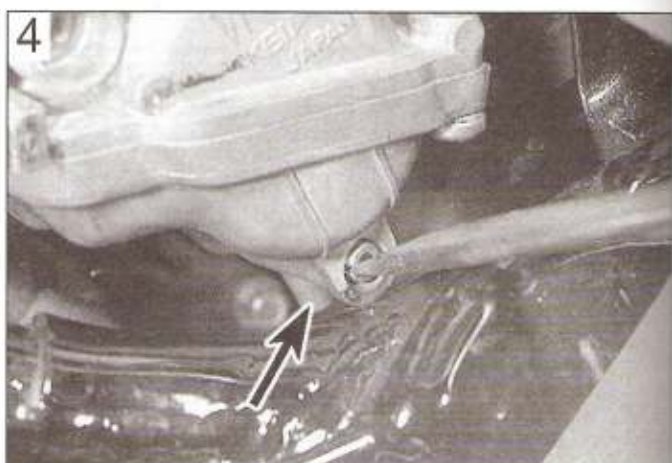
4 Connect a hose to the carburettor float chamber drain stub (arrow) and unscrew the drain screw
