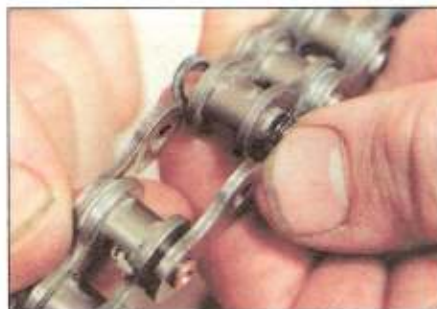
8.3 . . . and separate the chain link
