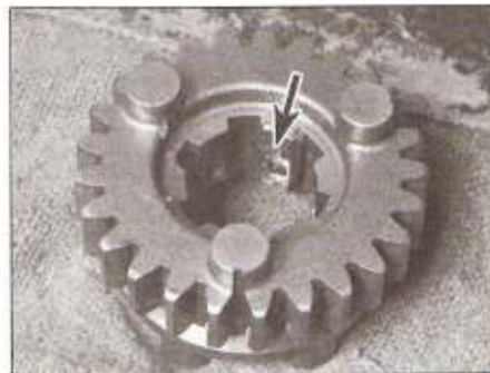
30.17k ... must align with the balls in fifth gear (arrowed) when it's installed
