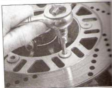
4.6 Loosen the disc retaining bolts a little at a time to prevent distortion
