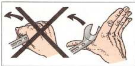
4.6 If you can't pull on the spanner to loosen a fastener, push with your hand open
