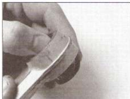
10.4 Push the sleeve out of the end of the tie-rod and remove the O-rings
