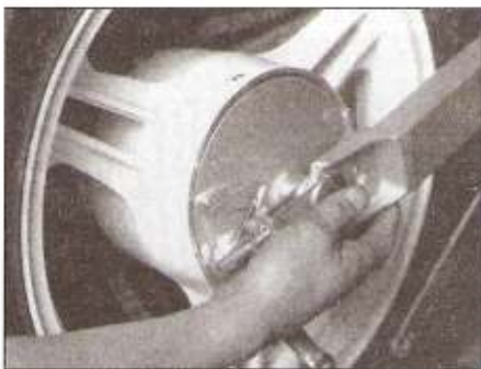
13.7 Slide the wheel rearward, set the chain adjuster down and pull the wheel the rest of the way out
