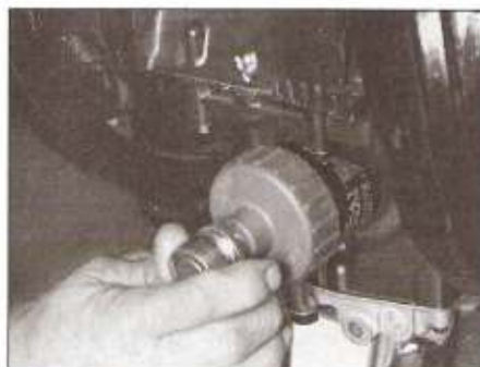
20.5a Remove the oil filter with a special adapter like this or a strap wrench
