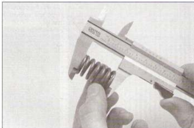
19.11 Measure the clutch spring free length
