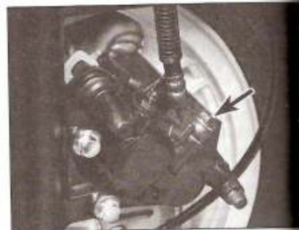
3.2 Remove the caliper hose banjo fitting bolt - there's a sealing washer on each side of the fitting
