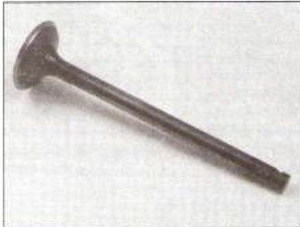
12.18 Check the valve face, stem and keeper groove for signs of wear and damage
