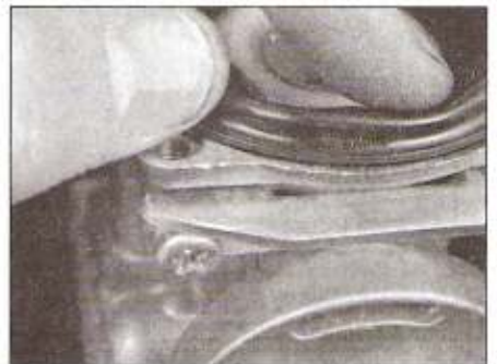
8.8 Make sure the bead of the vacuum diaphragm seats in its groove, and that the diaphragm isn't distorted
