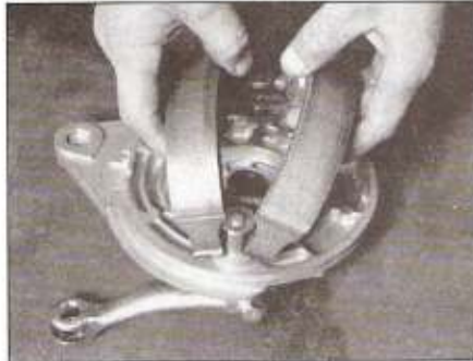
9.4 Fold the shoes off the panel to remove them
