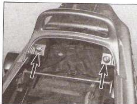
8.11 Remove the grab rail bolts (arrowed)
