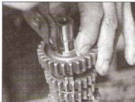
30.4d . . . remove the circlip and toothed washer, then slide off sixth gear . . .
