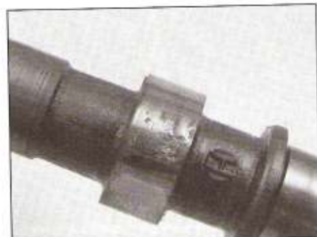
9.10a Check the lobes of the camshaft for wear – here's a good example of damage which will require renewal
