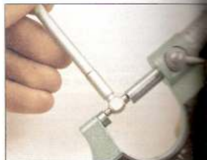
3.8 ... then measure the gauge with a micrometer
