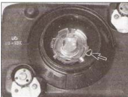
8.3 The bulb is held in place by this retaining clip
