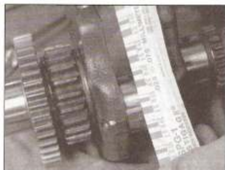
25.15 Measuring the width of the crushed Plastigauge (be sure to use the correct scale – standard and metric are included)
