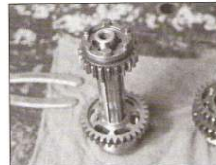
30.17c Install sixth gear with its fork groove away from second gear
