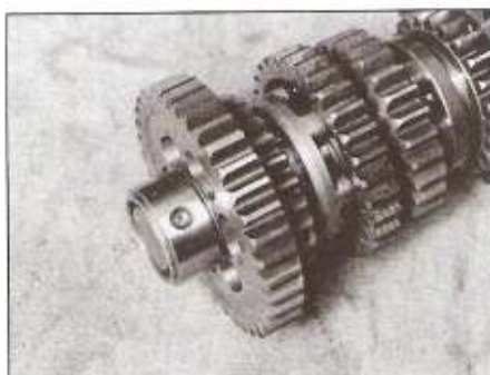
30.15a Pull off the bearing outer race ...
