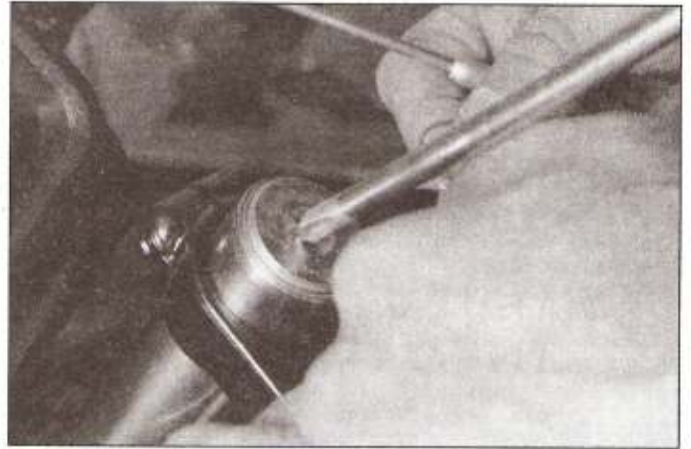
31.3b Release the spring tension on the top plug
