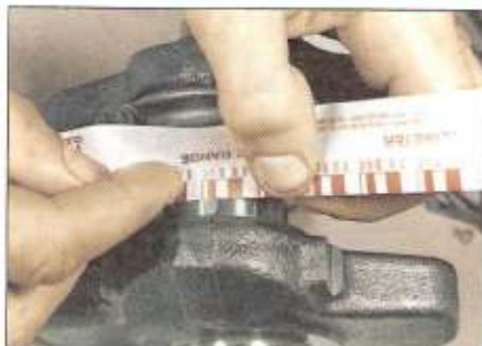
3.16 Measuring the width of the crushed Plastigauge
