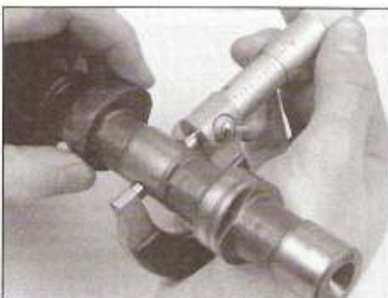
9.15b Measure the cam bearing journal with a micrometer
