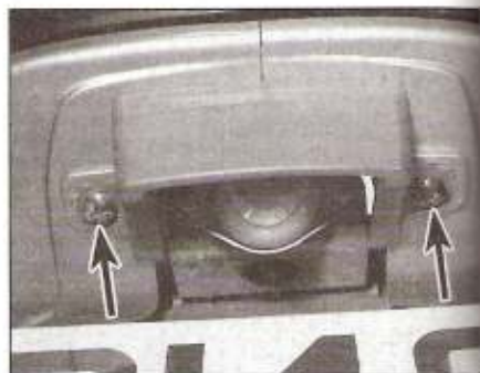
8.12c Licence plate light cover screws (arrowed)
