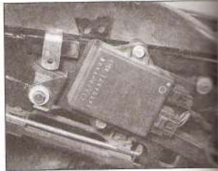
5.2b IC igniter location – EX500D and E
