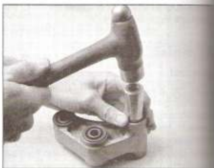
10.16b . . . then drive the new ones in with a socket that just fits into the bore of the rocker arm
