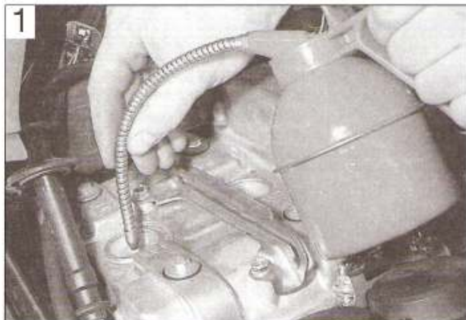
1 Squirt a drop of motor oil into each cylinder
