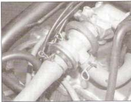
13.1 Location of the air switching valve
