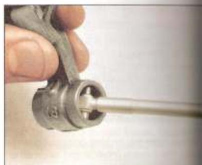
3.7 Expand the telescoping gauge in the bore, lock its position ...
