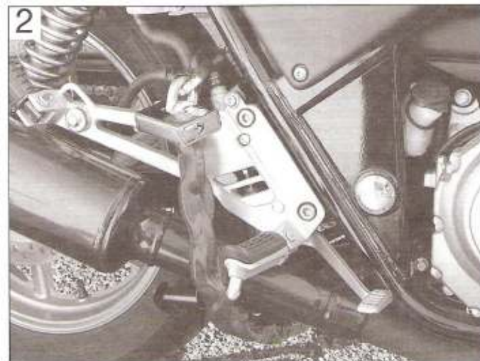
2 Pass the chain through the bike's frame, rather than just through a wheel ...
