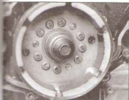
33.3 The alternator rotor bolt has left-hand threads (turn it clockwise to loosen it)
