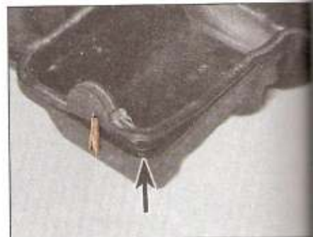
7.11a Be sure the gasket seats securely in the groove (arrowed)
