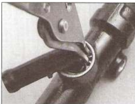
6.12 Remove the circlip which secures the hose union
