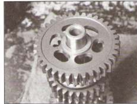
30.17l Install first gear and its spacer ...
