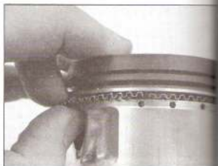
15.9a Installing the oil ring expander – make sure the ends don't overlap
