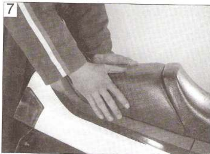
Bounce the rear of the motorcycle to check rear suspension operation
