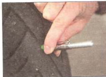
2 Measure tread depth at the centre of the tyre using a tread depth gauge.
