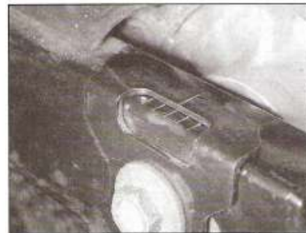
2.11b Chain adjuster plate notch and wheel alignment marks
