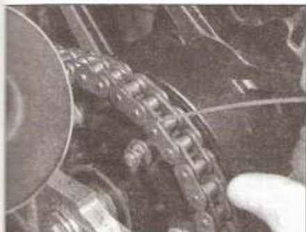
1.2 Apply chain lubricant to the joints between the side plates and the rollers – not in the centre of the rollers
