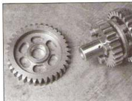
30.15c Slide first gear off the shaft
