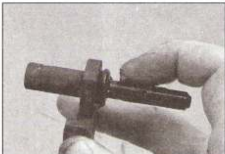
3.17 Apply a thin coat of the specified grease to the slider pins on the caliper bracket
