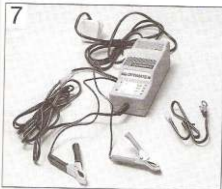
Use a suitable battery charger - this kit also assess battery condition
