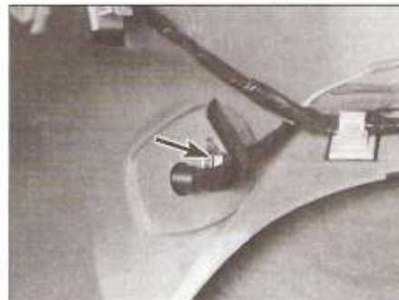
12.3 The turn signals are secured by a nut (arrowed) inside the fender or fairing
