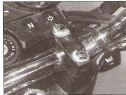
5.8a Arrow mark on clamp must face forwards
