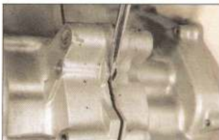
7.1 If a pry point is provided, apply gently pressure with a flat-bladed screwdriver
