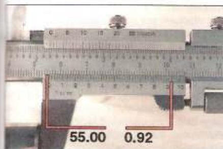
3.12 Vernier gauge reading of 55.92 mm
