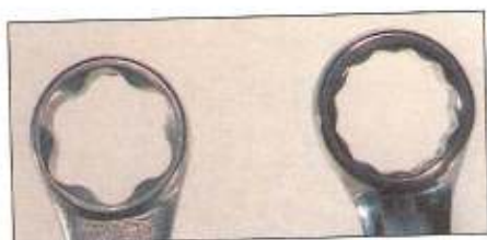
2.21 Comparison of surface drive ring spanner (left) with 12-point type (right)
