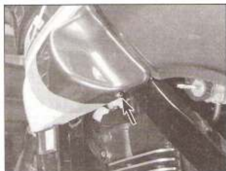
3.6 Remove the screw from under the fairing on each side (arrowed)
