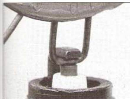
3.6a Spark plug manufacturers recommend using a wire type gauge when checking the gap
