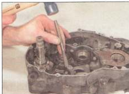
2.16 Using a hammer and chisel to free a seized fastener
