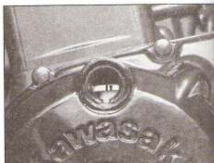
19.6b . . . until the T mark on the rotor aligns with the timing notch . . .
