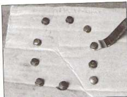
16.5b Place the bolts in a holder, such as a piece of cardboard with holes punched in it
