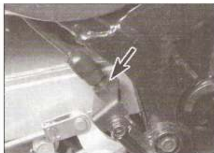
10.6 To adjust the rear brake light switch, hold the switch body and turn the adjusting nut (arrowed)
