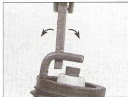
3.6b To change the gap, bend the side electrode only, as indicated by the arrows
