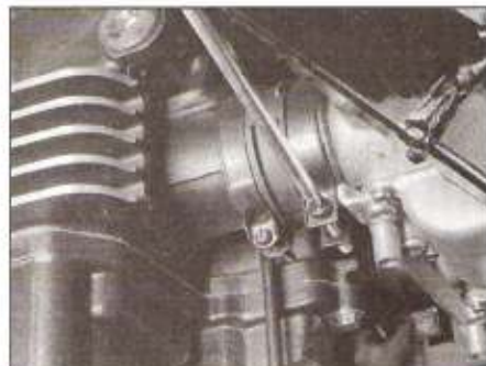
6.5 Loosen the clamps on the intake manifold tubes
