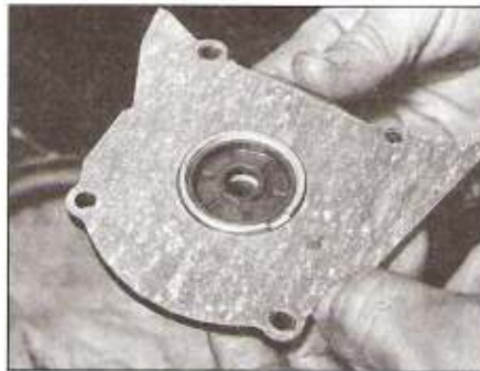
8.18 Install a new oil seal and gasket
