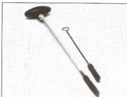
6.2a A selection of brushes is required for cleaning holes and passages in the engine components
