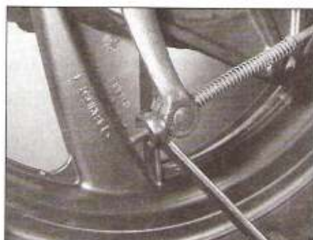
13.29a Unscrew the adjuster nut from the end of the brake rod
