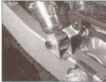
9.10c Shock lower mounting bolt on left side
