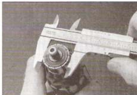
27.7 Check the commutator for cracks and discoloring, then measure the diameter and compare it with the minimum diameter listed in this Chapter's Specifications
