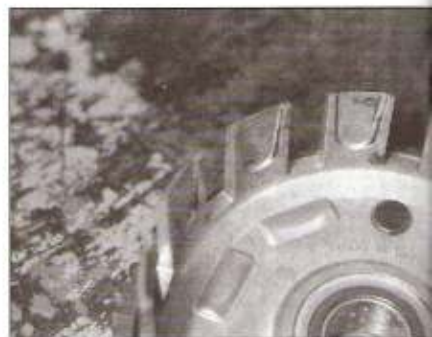
19.15 Check the slots on the clutch hub for indentations – if they're worn, the crankcase will have to be disassembled to remove the clutch hub
