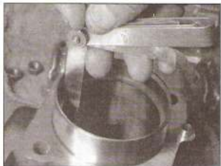
15.3b . . . then check the piston ring end gap with a feeler gauge
