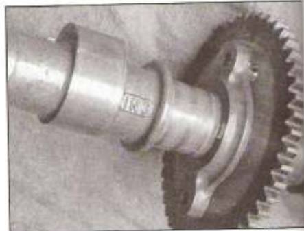
9.7b The camshafts are identified by punch marks
