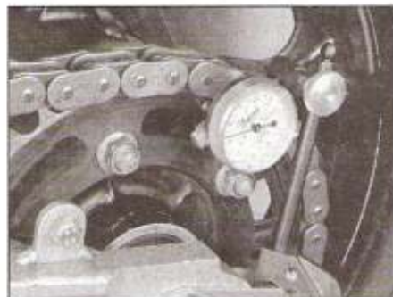
15.4 Check the runout of the rear sprocket with a dial gauge
