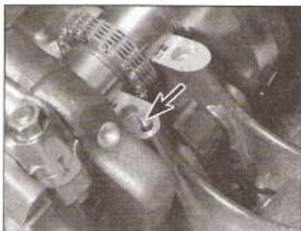
23.6a Remove this lock-pin if you plan to remove the cam chain tensioner blade ...
