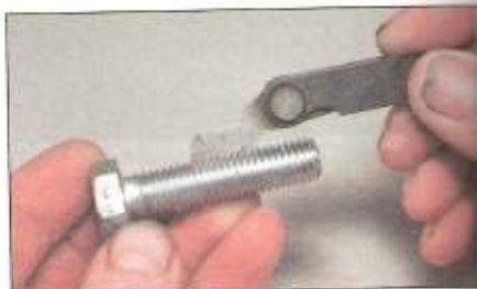
2.12 Using a thread gauge to measure pitch
