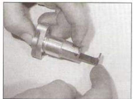
8.20 Release the ratchet and press the plunger into the body
