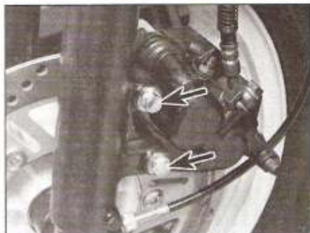
2.2a Remove the front caliper mounting bolts (arrowed) and support the caliper so it doesn't hang by the brake hose
