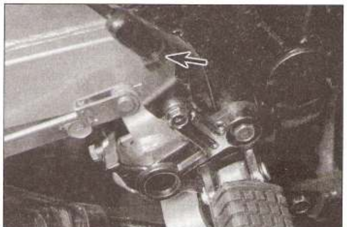
14.10 Loosen the adjuster nut (arrowed) and unscrew the switch
