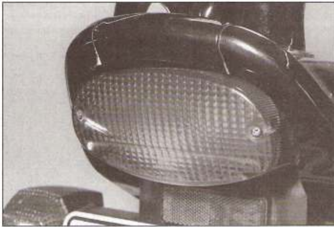
11.12 The lens is retained by two screws
