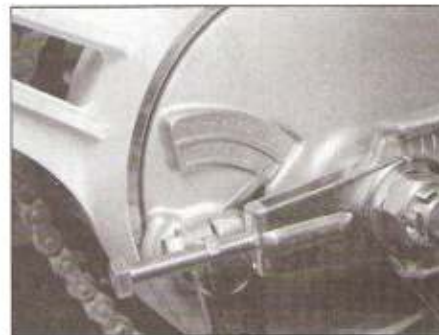
11.4 If the pointer goes past the Usable Range indicator toward the rear of the bike, the linings are worn and must be renewed
