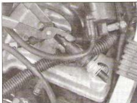
2.3 With the wire attached, ground a spark plug to the engine and operate the starter - bright blue sparks should be visible
