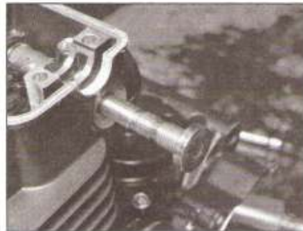
9.30b . . . unscrew the shaft and pull it out
