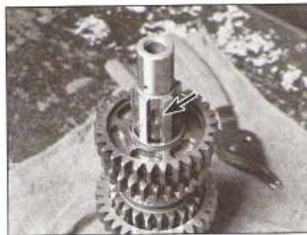
30.15f ... which locate in these slots (arrowed)
