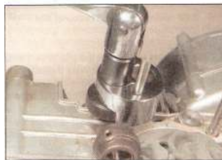
2.17 Using a stud extractor tool to remove a broken crankcase stud
