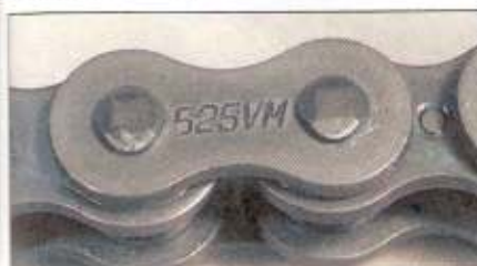
8.10 Typical chain size and type marking
