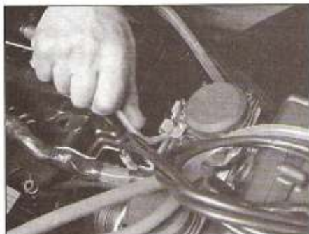
10.2 Separate the choke cable housing from the bracket at the carburettor
