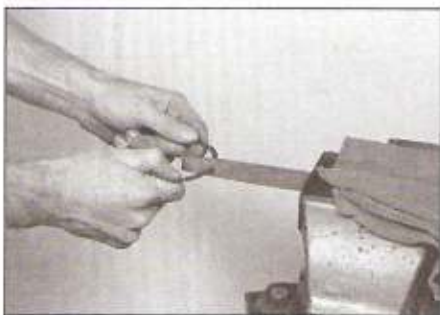
15.5 If the end gap is too small, clamp a file in a vice and file the ring ends (from the outside in only)
