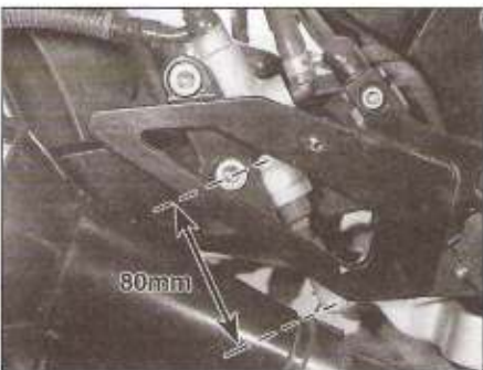
6.19 Distance from centre of lower mounting to centre of clevis pin must measure 80 mm
