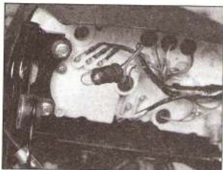
17.2 Pull the bulb socket out of the cluster, then pull the bulb out of the socket
