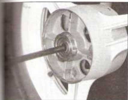
14.22 Insert a drift into the hub and tap evenly around the opposite bearing to drive it out
