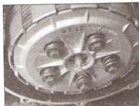
19.6b When spring tension is released, remove the springs and the spring plate
