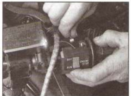
9.12 Hold the rear half of the housing in place and install the accelerator cable
