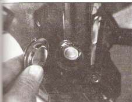
12.4a Remove the plastic cap from the pivot shaft head . . .
