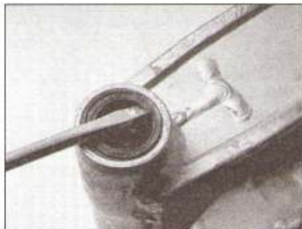
13.4 Pry the seals out with a screwdriver
