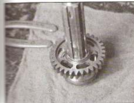
30.17b . . . and install second gear (flat side toward bearing), then secure it with a toothed washer and circlip
