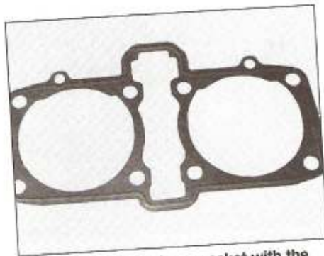
13.14 Install the base gasket with the ridge upward
