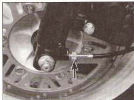
12.2 Unscrew the speedometer cable nut (arrowed)
