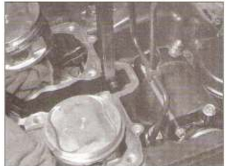
13.4 Lift the rear cam chain guide out of the engine (cylinder block removed for clarity)
