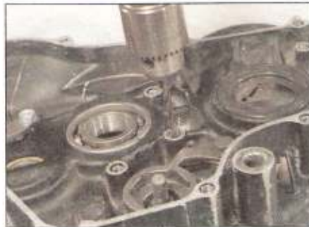
2.19 When using a screw extractor, first drill a hole in the fastener . . .
