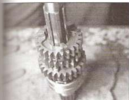
30.11c Install the third-fourth gear cluster with third gear (the smaller gear) toward fifth gear
