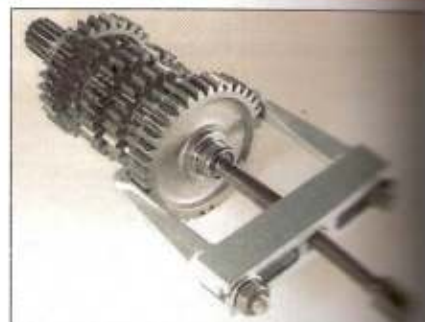
5.4 Where no access is available to the inner of the bearing, it is sometimes possible to draw off the adjacent component
