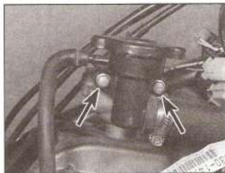
6.5b Unbolt the thermostat housing from the filler neck
