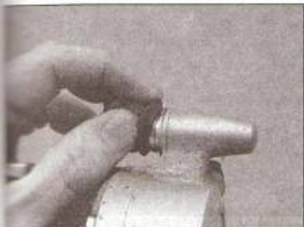
3.16 Install the slider pin boots
