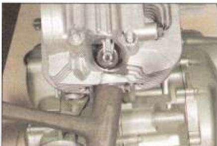
7.2 Tap around the joint with a soft-faced mallet if necessary - don't strike cooling fins
