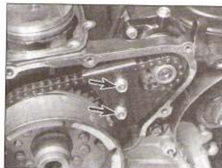
26.5 Remove the starter chain cover bolts (arrowed)
