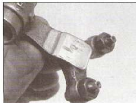
9.33 Inspect the rocker arms, especially the faces that contact the cam lobes, for wear
