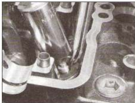
12.7b Remove the valve keepers/collets with needle-nose pliers or tweezers
