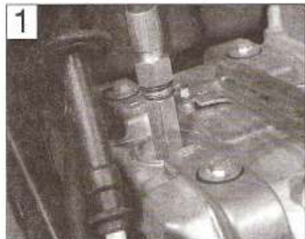
Screw the compression gauge adapter into the spark plug hole, then screw the gauge into the adapter
