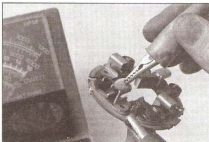
27.10 There should be no continuity between the brush plate and the brush holders (the resistance should be infinite)
