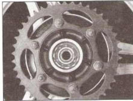
14.13 Pry the grease seal out of the sprocket coupling
