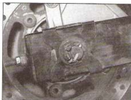
13.25 Make sure that the axle nut is secured correctly
