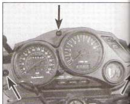
15.2b On the EX500D/E, remove the trim screws (arrowed) and withdraw the trim panel . . .
