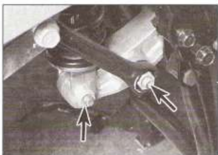
9.4 Remove the shock absorber lower nut and bolt (left arrow) and tie-rod nut and bolt (right arrow)
