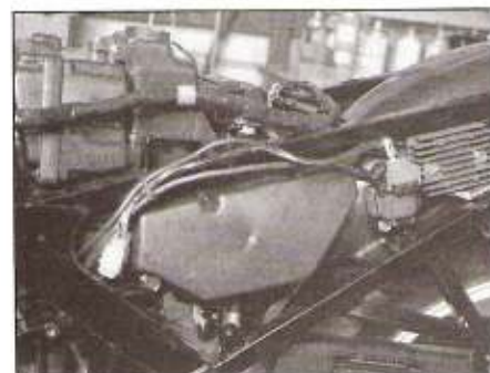
11.5 The housing side covers are secured by screws
