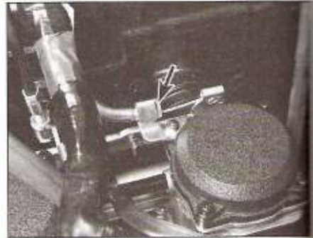
10.6 The cable housing should be securely seated in the bracket
