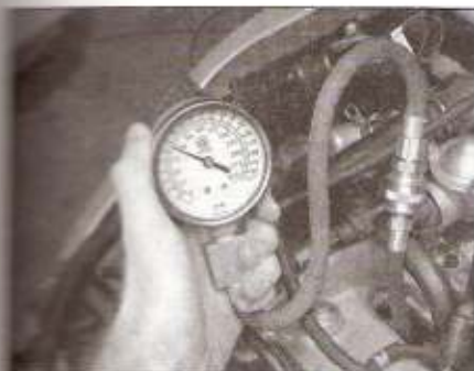
35.2 A compression gauge with a threaded fitting for the spark plug hole is recommended
