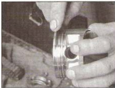
14.13 Measure the piston ring-to-groove clearance with a feeler gauge
