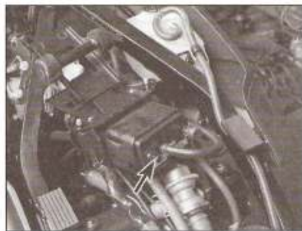
7.6b ... disconnect the purge hose from the canister fitting (arrowed) (the other canister hose can be left connected and the canister-to-tank bracket bolts can be left in place) ...
