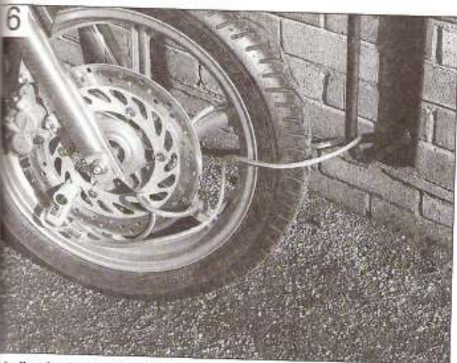
6 A disc lock combined with a security cable provides additional protection
