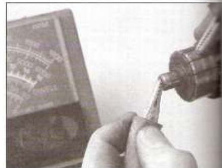
27.8b There should be no continuity between the commutator bars and the armature shaft
