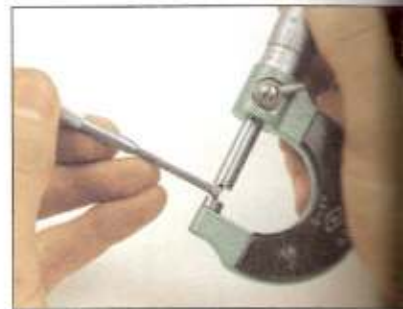
3.10 ... then measure the gauge with a micrometer
