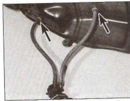
22.8b Fuel filter unions on ER models (arrowed)
