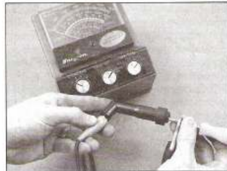
2.5 Unscrew the spark plug caps from the plug wires and measure their resistance with an ohmmeter
