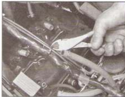
9.2 Cut the tie wrap that secures the cables to the wiring harness
