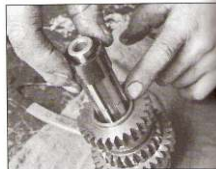
30.15j ... slide off the bushing and fourth gear
