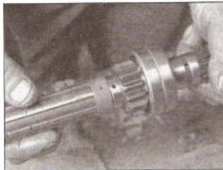
30.11a If the main drive shaft fifth gear has a separate bushing, install it so its oil hole lines up with the hole in the shaft
