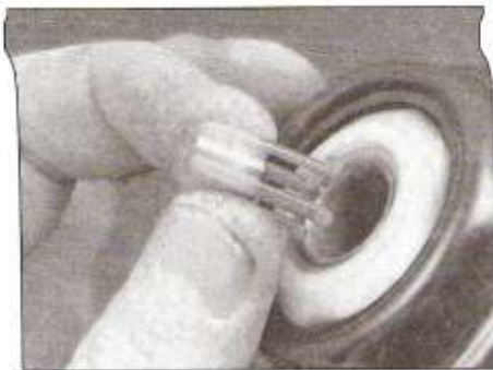
7.5a Remove the vacuum piston spring seat from the piston
