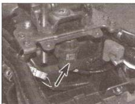
7.4a Location of the headlight relay (arrowed)
