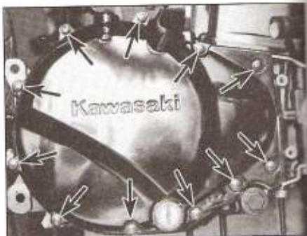
19.5a Remove the clutch cover bolts (arrowed) . . .
