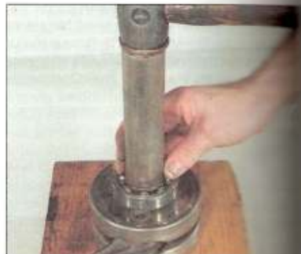
5.5 When installing a bearing on a shaft, use a piece of tubing which bears against the bearing's inner race
