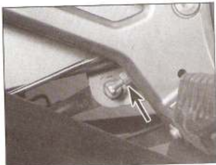
12.2b Brake pedal position bolt locknut (arrowed) – ER models
