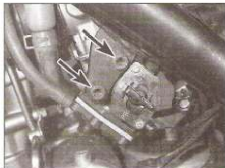
2.10a The fuel tap is retained by two bolts (arrows)
