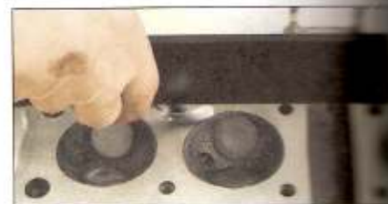
3.22 Use a straight-edge and feeler gauges to check for warpage
