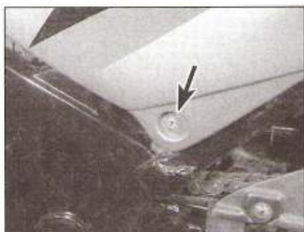
8.12a Side cover retaining screw (arrowed) at the front ...
