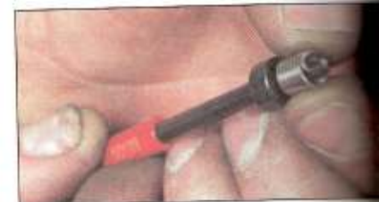
2.28 ... fit insert on the installing tool
