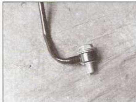
10.20 Use a new washer on each side of the oil line banjo bolt fittings
