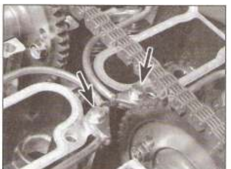
9.5 Remove the oil line bolts (arrowed) and lift the oil pipes and O-rings out of the engine
