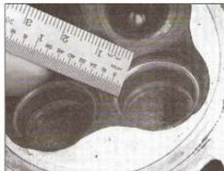
12.15 Measuring the valve seat width
