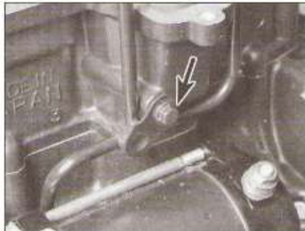
13.3 If you haven't already done so for cylinder head removal, remove the oil pipe mounting bolt
