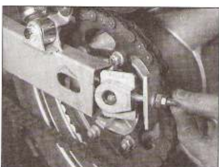
13.33 Make sure the chain adjusters are in place in the swingarm ends
