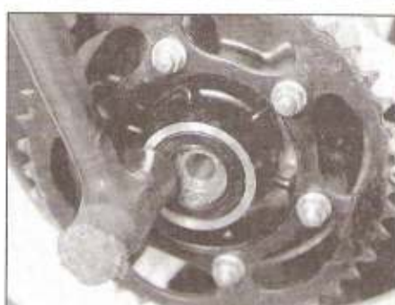
14.19 Tap a new grease seal in evenly
