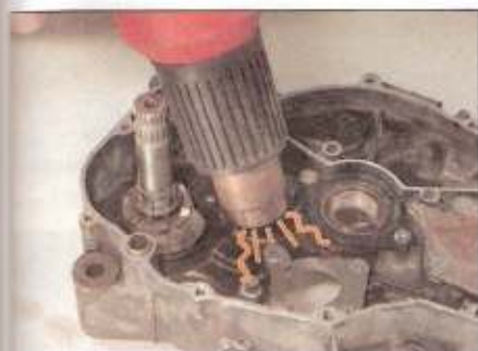
2.15 Using heat to free a seized fastener
