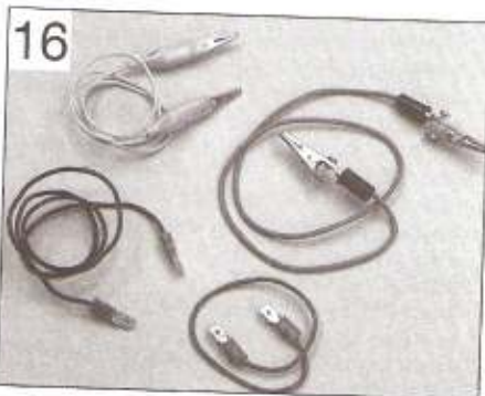
16 A selection of jumper wires for making earth (ground) checks
