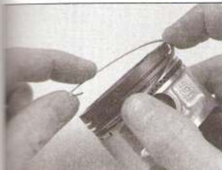
15.9b Installing an oil ring side rail – don't use a ring installation tool to do this
