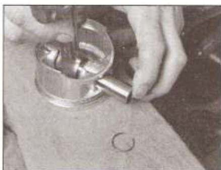
14.15 Slip the pin into the piston and try to wiggle it back-and-forth; if it's loose, renew the piston and pin
