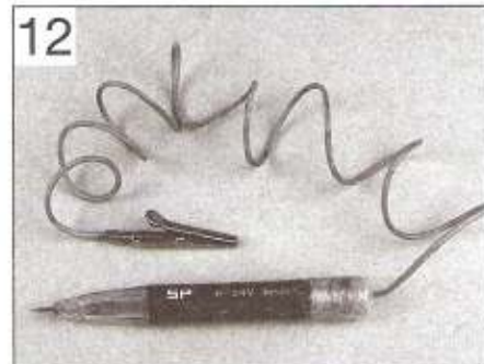
12 A simple test light can be used for voltage checks
