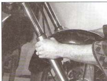
16.4 Check for freeplay in the steering head bearings
