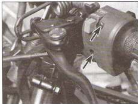
10.3 The choke cable/switch housing is held together by screws (arrowed)
