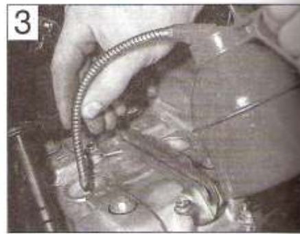
Bores can be temporarily sealed with a squirt of motor oil
