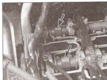
19.6c . . . and the no. 1 cam lobes point upward
