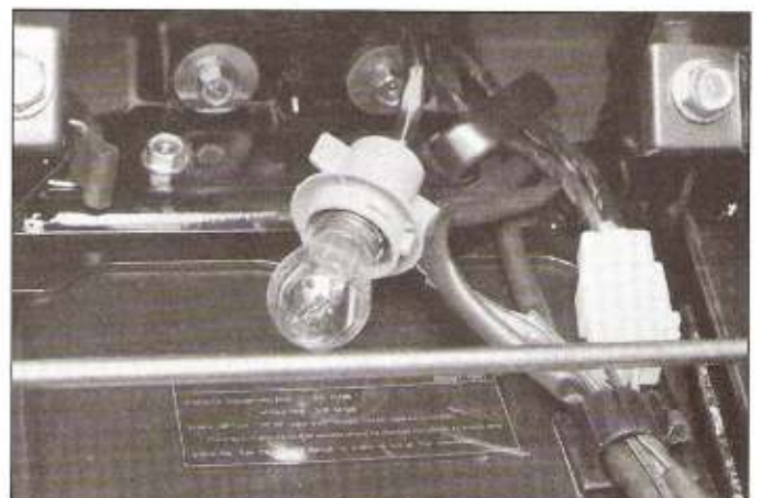
11.8b . . . then rotate the holders and pull them out of their sockets
