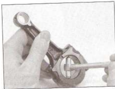
26.20a Assemble the connecting rod and measure the diameter of the bore with a telescoping gauge – then measure the gauge with a micrometer.
