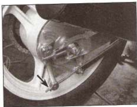
12.4 Turn the adjuster at the rear of the brake rod (arrowed) to adjust pedal freeplay
