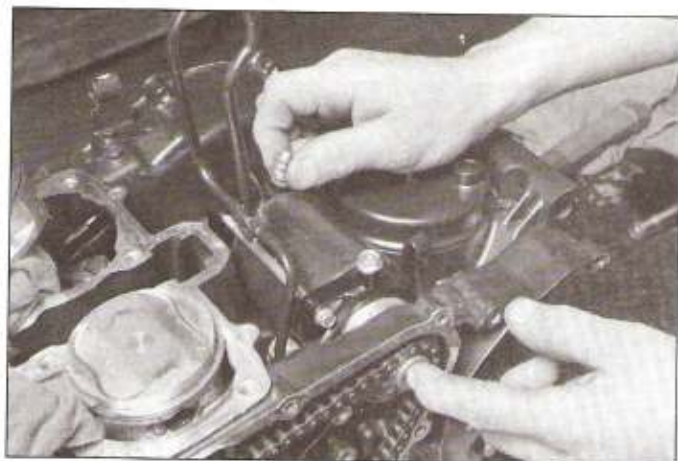
26.7 Lift the starter and disengage it from the chain
