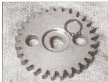
17.16 The recessed side of the drive gear faces away from the oil pump – the circlip fits into the recess
