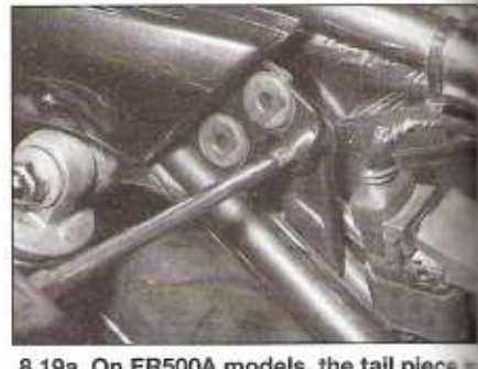
8.19a On ER500A models, the tail piece is retained by a screw at each forward end (arrowed) ...
