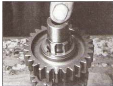
30.11h . . . then secure the gear and washer with a circlip
