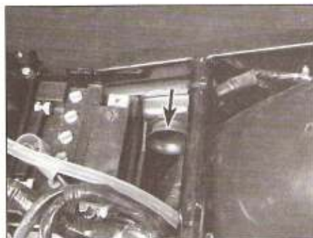
6.14b . . . and be careful not to place its end near the air intake (arrowed); this will cause fuel starvation
