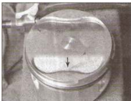
14.3 Using a sharp scribe, scratch the cylinder numbers into the piston crowns – also note the arrow, which must point to the front
