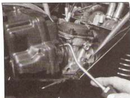
6.7a Pull the spring bands back, toward the air cleaner housing – EX models
