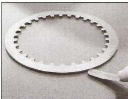
19.13 Check the metal plates for warpage
