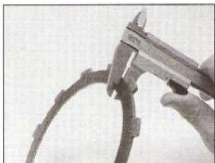
19.12 Measure the thickness of the friction plates
