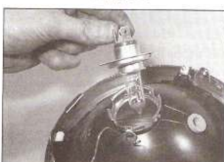
8.9b . . . and lift the bulb out of the headlight
