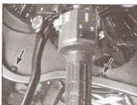
3.3 Remove the screws (arrowed) and detach the inner fairing on each side of the motorcycle
