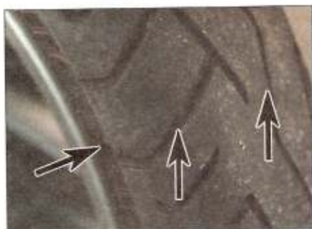
3 Tyre tread wear indicator bar and its location marking (usually either an arrow, a triangle or the letters TWI) on the sidewall (arrowed).
