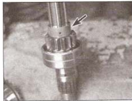
30.4j ... and the fifth gear bushing (if equipped)
