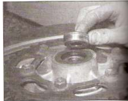
13.21 Insert the left-hand spacer in the hub
