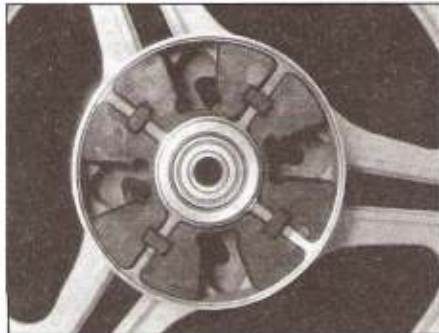
16.5 The damper should look like this when it's installed
