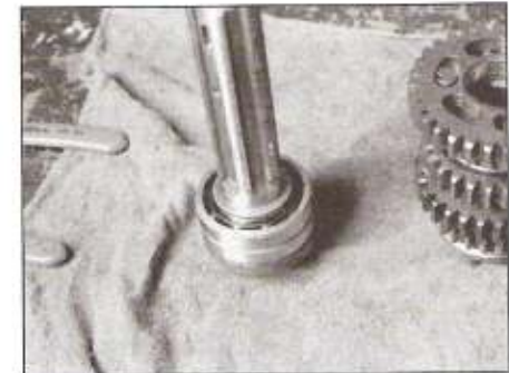
30.17a Stand the shaft on its ball bearing end . . .
