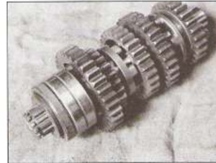
30.17o ... don't forget the seal on the other end of the shaft
