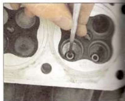
3.9 Expand the small hole gauge in the bore, lock its position ...
