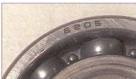
5.16 Typical bearing marking
