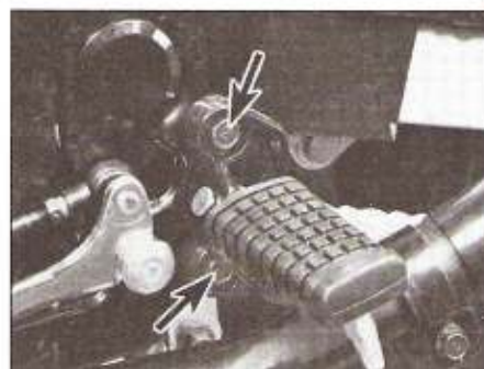
3.8 The rider's left side footrest bracket is secured by two bolts (arrowed)
