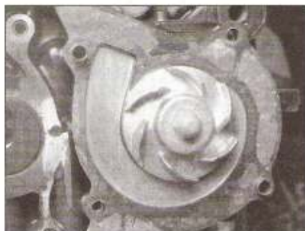
8.6 If you can wiggle the impeller or pull it in-and-out, the pump is defective
