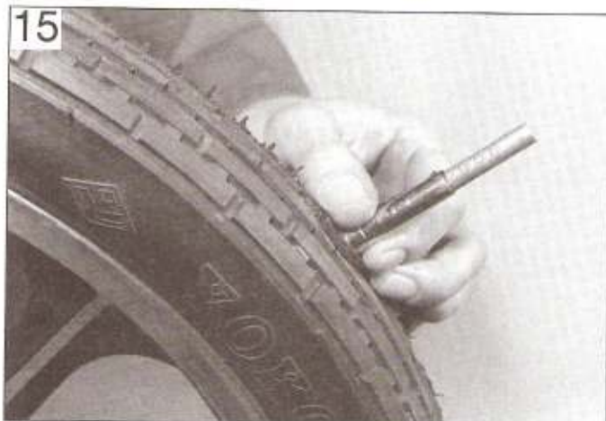
Checking the tyre tread depth
