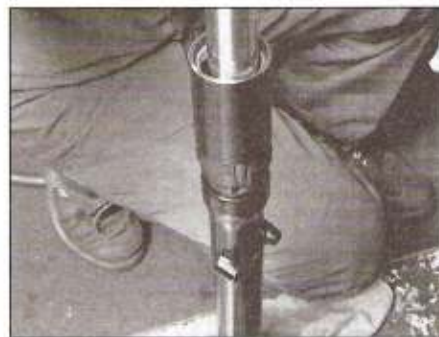
7.20b . . . then use a seal driver to seat it in the outer fork tube
