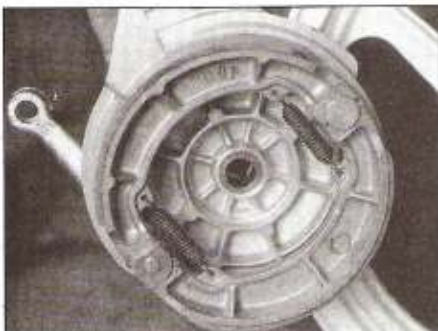
9.3 The brake shoes are mounted on a panel that fits into the rear wheel
