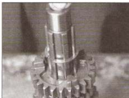
30.11d Install a circlip in the next shaft groove . . .
