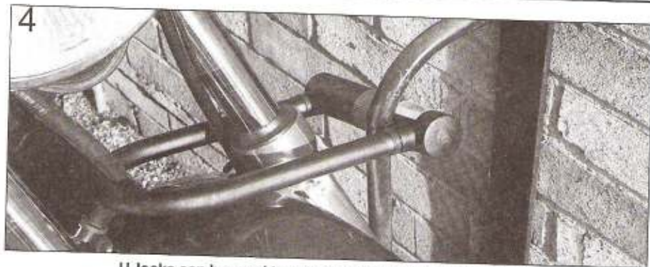
4 U-locks can be used to secure the bike to a solid object – ensure you purchase one which is long enough
