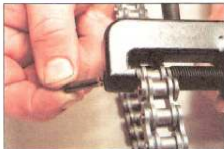
8.2 . . . withdraw the pin, remove the tool . . .
