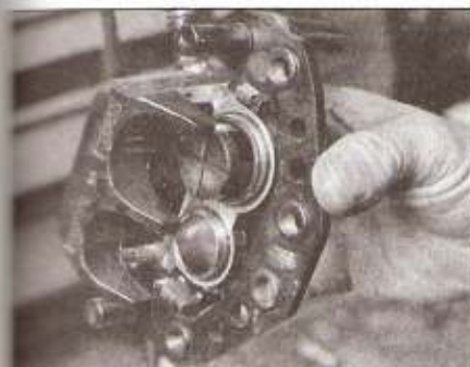
3.5 Remove the insert from each piston
