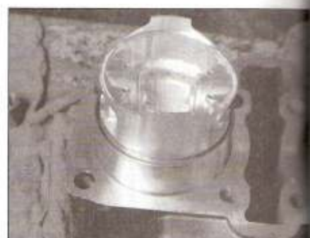
15.3a Square the ring in the bore by turning the piston upside down and tapping on the ring . . .
