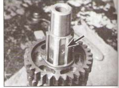
30.17j ... and secure them with a circlip; the slots in the shaft (arrowed) ...
