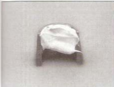
12.27 A small dab of grease will help hold the keepers/collets in place on the valve spring while the valve is released
