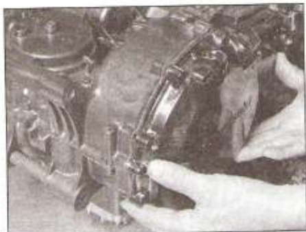
19.5b . . . take the cover off (tap it gently with a soft-faced hammer if it's stuck) . . .
