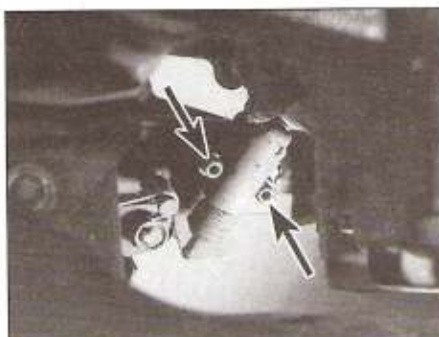
23.7 The sidestand switch is retained by two screws on ER models
