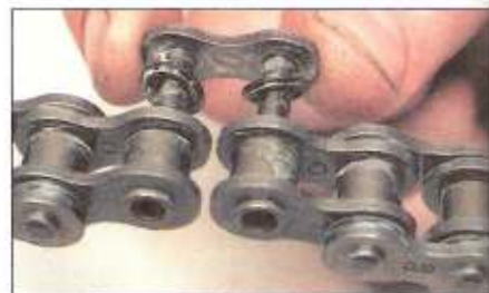
8.4 Insert the new soft link, with O-rings, through the chain ends . . .
