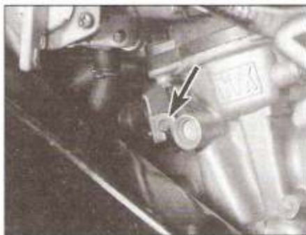
18.10a Operate the choke lever until the linkage shaft and plunger touch ...
