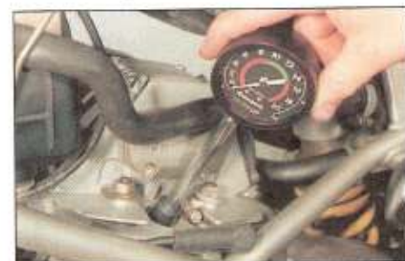
3.20 Using a rubber-cone type cylinder compression gauge
