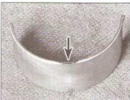
25.16 Bearing thicknesses are identified by colour codes on the sides of the bearings
