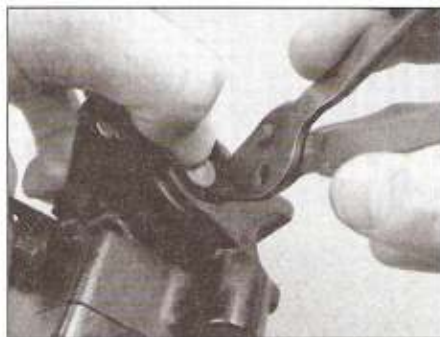
5.10a . . . then depress the piston and remove the circlip with a pair of circlip pliers
