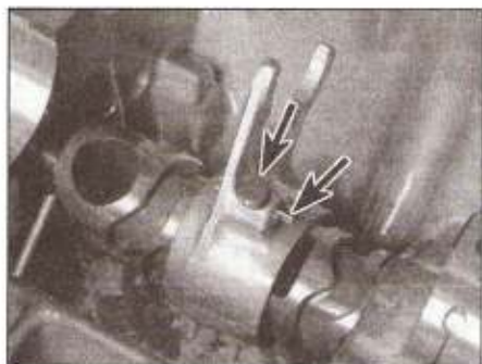
31.4 Remove the cotter pin (split pin) and guide pin (arrowed) . . .
