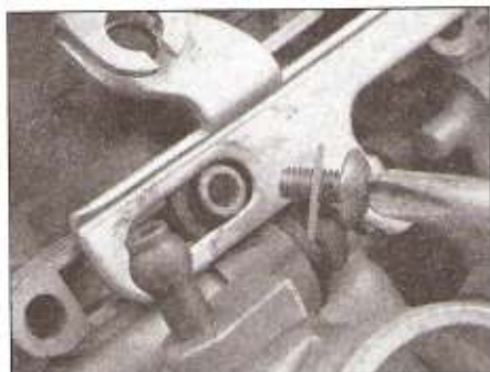
8.15 Make sure to install a plastic washer on each side of the choke linkage rod when installing the screws
