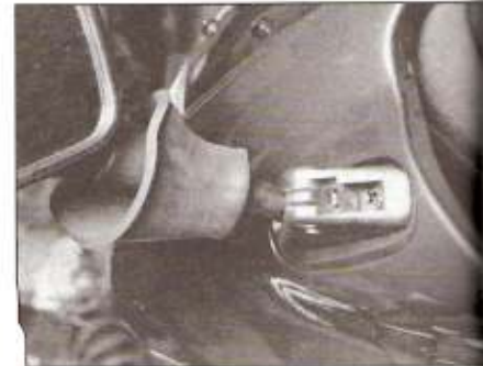
5.1 Pull back the rubber cover and remove the mirror mounting screws
