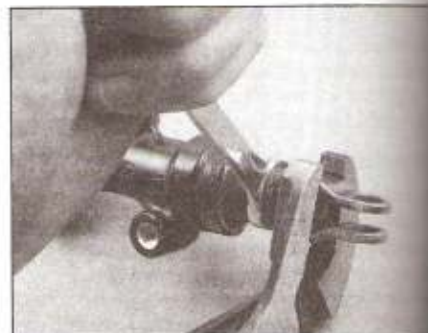
6.7b Hold the clevis and slacken the locknut
