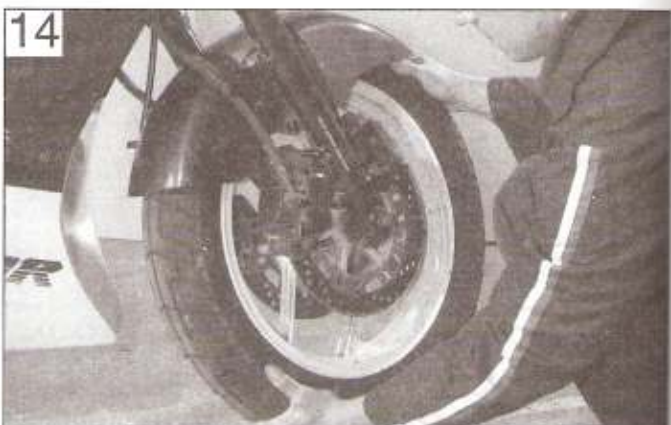
14 Check for wheel bearing play by trying to move the wheel about the axle (spindle)
