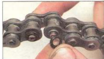
8.5 . . . install the O-rings over the pin ends . . .
