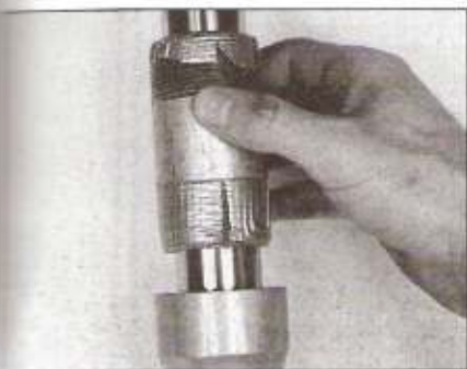
7.18b If you don't have the proper tool a section of pipe can be used as a driver
