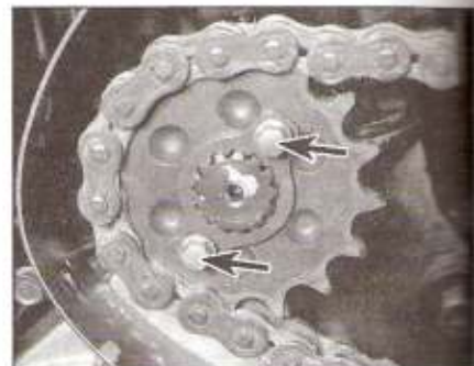
15.6a Remove the engine sprocket holding plate bolts
