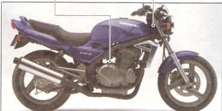
The engine number is stamped into the top of the crankcase on the right-hand side of the engine.
