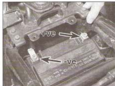
3.10 Battery negative (-ve) cable and positive (+ve) cable
