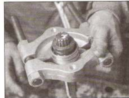
30.15q If the bearing is worn or damaged, place it in a bearing splitter, press it off the shaft and press a new one on (or have the job done by a motorcycle dealer)
