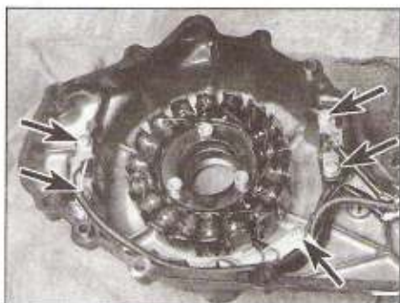
4.6a Pick-up coil screws (upper arrows) and wiring clip (lower arrow) – EX500A
