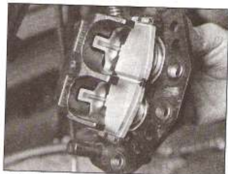
2.4b Disengage the clips on the outer pad from the caliper and remove the pad
