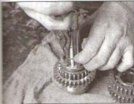
30.15k Remove the toothed washer, then the circlip . . .
