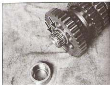
30.15b ... the bearing and spacer (arrowed)
