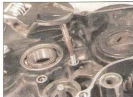
2.20 . . . then thread the extractor anti-clockwise into the fastener
