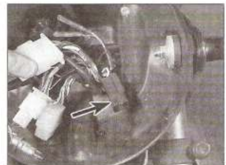
6.18 Coolant temperature warning light diode (arrowed)
