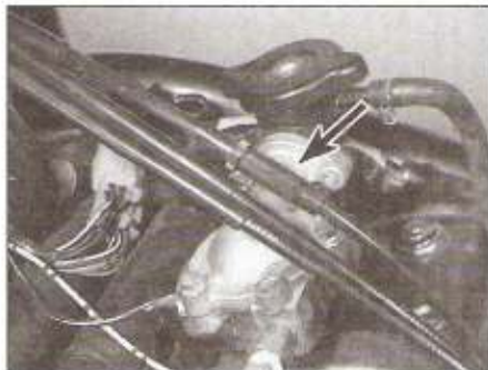
18.11b Choke cable adjuster (arrowed) on ER models
