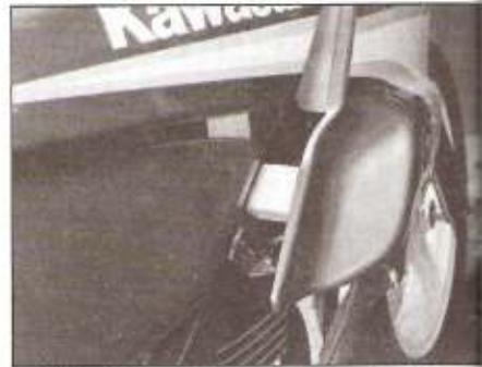
3.7b If you only need access to other components, you can prop the fairing away from the sides of the bike with blocks of wood
