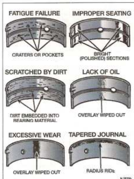
5.17 Typical bearing failures
