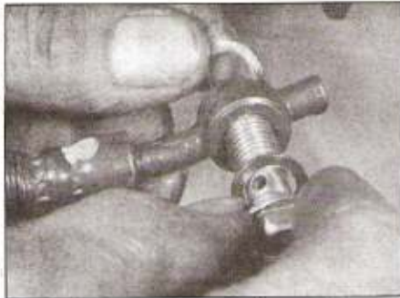
7.4 Always use a new sealing washer on each side of the banjo union
