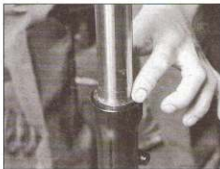
7.20a Press the oil seal into the fork outer tube as far as you can with finger pressure . . .
