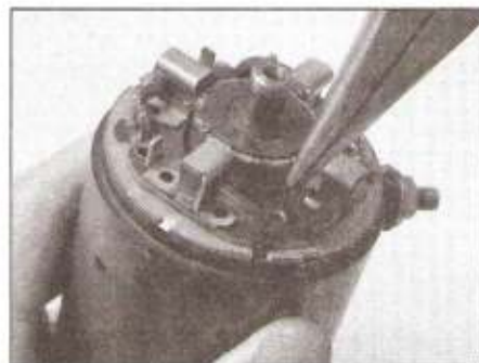
27.14b . . . then pull the end of the spring 1/2 turn clockwise and seat the end of it in the groove in the end of the brush
