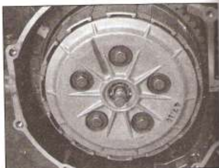
19.6a Loosen the spring bolts in a criss-cross pattern . . .
