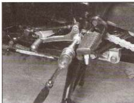
21.2 Remove the gearchange pedal Allen bolt
