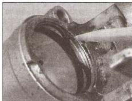
3.9 The dust seal and fluid seal should be carefully removed
