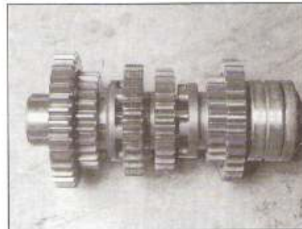
30.17n ... and the bearing outer race – the assembled output shaft should look like this ...
