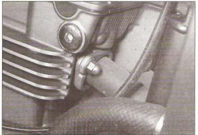
12.11 Remove the nuts and holders from the cylinder head
