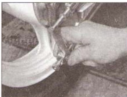
13.4 Remove the nut from the brake rod, then slip the rod out of the pin
