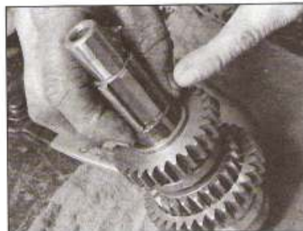
30.15i ... this will expose the bushing shared by third and fourth gears ...
