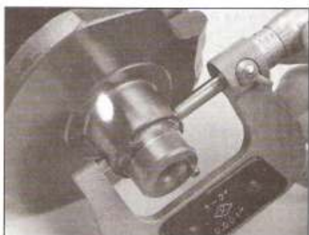
25.18 Measure the diameter of each crankshaft journal at several points to detect taper and out-of-round conditions
