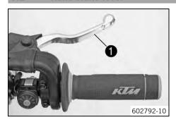
Hand brake lever **1** is located on the right side of the handlebar. The front brake is engaged using the hand brake lever.
