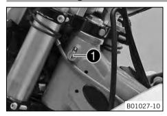
Steering lock  $\bullet$  is fitted on the left side of the steering head. The steering lock is used to lock the steering. Steering, and therefore riding, is no longer possible.
