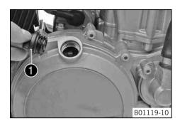
Remove the oil filler plug ● with the O-ring from the clutch cover and fill up with engine oil.
