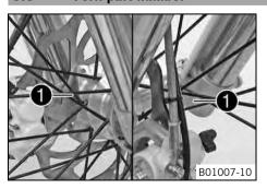
The fork part number **1** is stamped on the inner side of the axle clamp.
