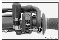
Electric starter button • is fitted on the right side of the handlebar.
