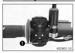
Turn signal switch lacktriangle is fitted on the left side of the handlebar.
