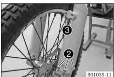
Position the fork protection on the left fork leg. Mount and tighten screws ②.
