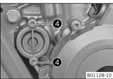
Remove screws 4. Remove the oil filter cover with the O-ring.
