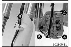
Position brake caliper, and mount and tighten screws 4.
