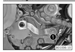
The engine number lacktriangle is stamped on the left side of the engine under the engine sprocket.
