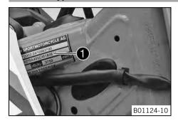
The type label **1** is fixed to the frame at the front right.
