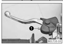
Adjust the basic position of the clutch lever to your hand size by turning adjusting screw •.
