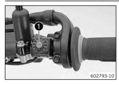
Electric starter button **1** is fitted on the right side of the handlebar.
