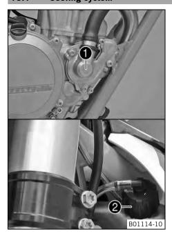
Water pump • in the engine circulates the coolant.
