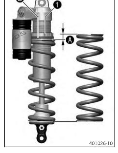
Depending on the static sag and/or the riding sag, it may be necessary to increase or decrease the spring preload.
