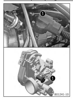
Idle speed adjusting screw **①** is located on the throttle valve body at the top left. The idle speed adjusting screw has two functions.
