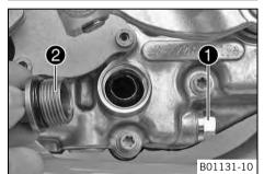
Mount and tighten screw plug ② with the O-ring.
