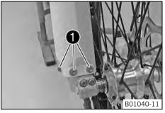
Position the fork protection on the right fork leg. Mount and tighten screws ①.
