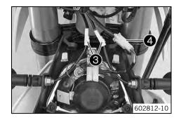
Disconnect the connectors of the turn signals 3 and headlight 4.
