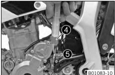
Fill bleeding syringe 4 with the appropriate hydraulic fluid.
