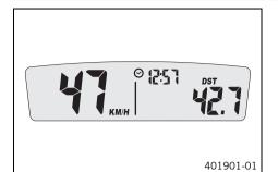
Press one of the buttons until **DST** appears on the speedometer.
