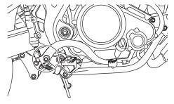
The operation of the brake pedal should be checked before each ride, and the pedal pivot should be lubricated if necessary.
