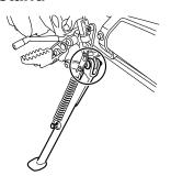
The operation of the sidestand should be checked before each ride, and the sidestand pivot and metal-to-metal contact surfaces should be lubricated if necessary.
