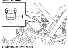
Insufficient brake fluid may allow air to enter the brake system, possibly causing it to become ineffective.
