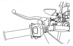
The operation of the brake and clutch levers should be checked before each ride, and the lever pivots should be lubricated if necessary.
