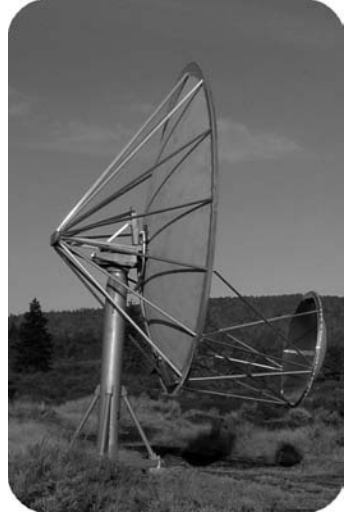
FIGURE 49-1 The ATA offset Gregorian optics before the addition of the feed and ground shield
