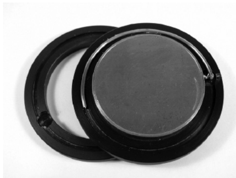
FIGURE 38-11 Circumference antenna on a pacemaker model (after A. Johansson, 169 Figure 5-3)
