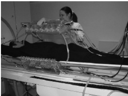
FIGURE 38-8 A prototype of the new Berlin MR-compatible Water-Coated Antenna Applicator (WACO) (after J. Nadobny et al. 137 © IEEE 2005)
