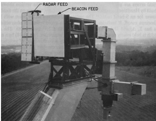
FIGURE 43-16 Integral beacon feed for the ARSR-3 (Courtesy of Westinghouse Electric Corp.)
