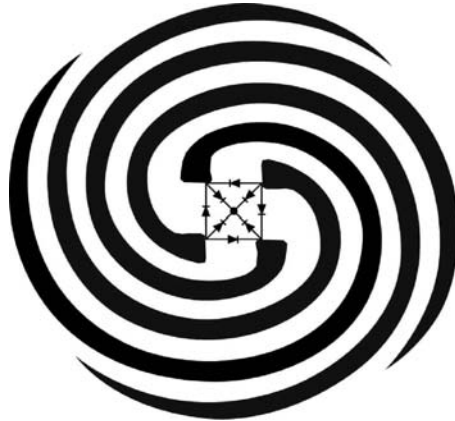
FIGURE 35-4 Reflectarray using a four-arm spiral element with switching diodes at center to achieve a 2-bit phase-shift system for circular polarization
