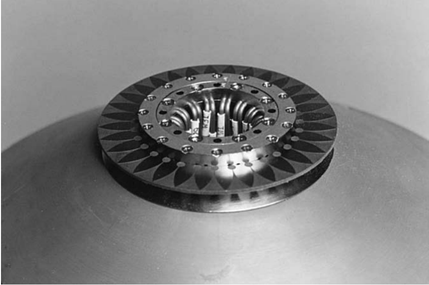
FIGURE 22-18 Circular array (Courtesy of Anaren Corporation)
