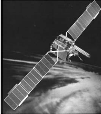
FIGURE 12-31 SKYNET 4 UK MOD spacecraft UHF helical antenna designed and built in 1984 by Sultan et al 61-63 at CAL (Canadian Astronautics Limited—now EMS Technologies Ottawa). Similar antennas were later deployed on NATO and The National Reconnaissance Office. GeoLITE satellite built by TRW/NRO, http://spaceflightnow.com/delta/d285/010517geolite.html . Posted May 17, 2001.
