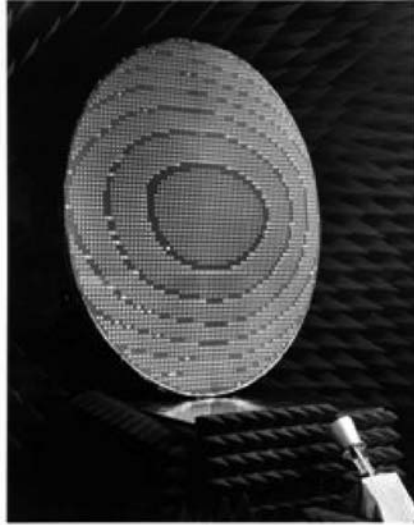
FIGURE 35-18 Ku-band reflectarray with shaped contour beam capability (Courtesy of Professor Dave Pozar, Univ. of Massachusetts)
