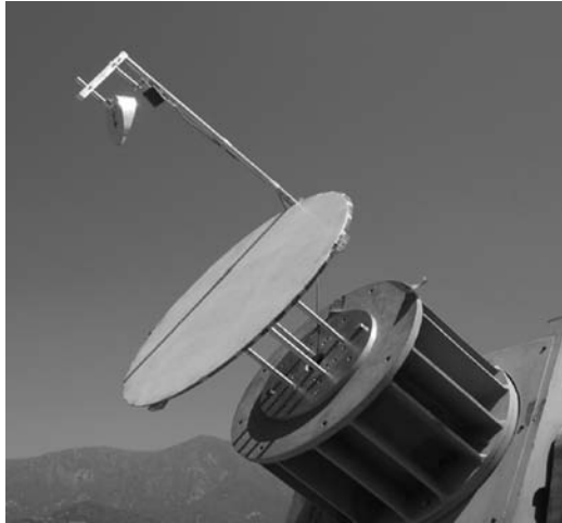
FIGURE 35-20 X/Ka dual-band Cassegrain reflectarray antenna (0.75-m diameter) using annular ring elements
