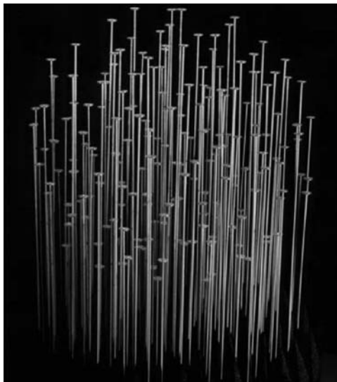
FIGURE 1-23 Volumetric array antenna with randomly distributed loop elements: Crow's nest antenna by FGAN e.V., Wachtberg, Germany 20 (Courtesy of FGAN e.V., Wachtberg, Germany)
