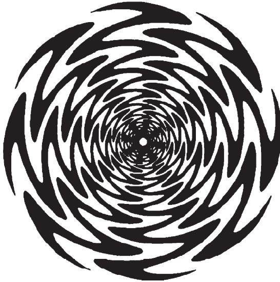
FIGURE 13-75 An eight-arm self-complementary sinuous antenna
