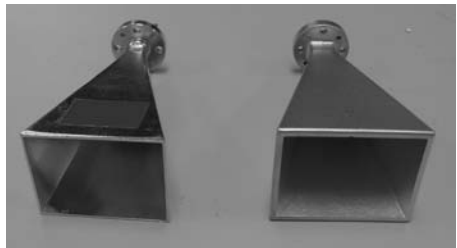
FIGURE 23-4 Horn antennas, connected to a WR15 waveguide, operating at millimeter-wave frequencies. The horn antenna on the left is precision assembled whereas the horn on the right is cast and plated for lower cost.
