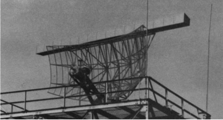
FIGURE 43-7 Typical hog-trough antenna (Courtesy of Department of Transportation, Federal Aviation Administration)
