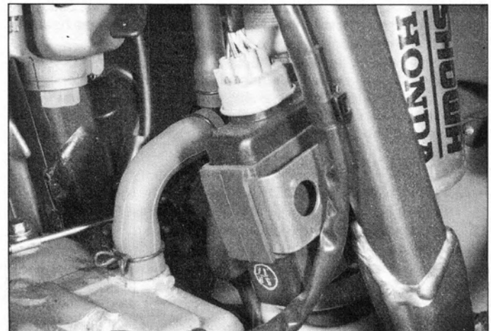
16.7 The XR400R ignition control module is in a mount on the frame
