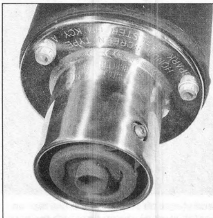
14.5a Remove the Allen bolts at the end of the muffler . . .
