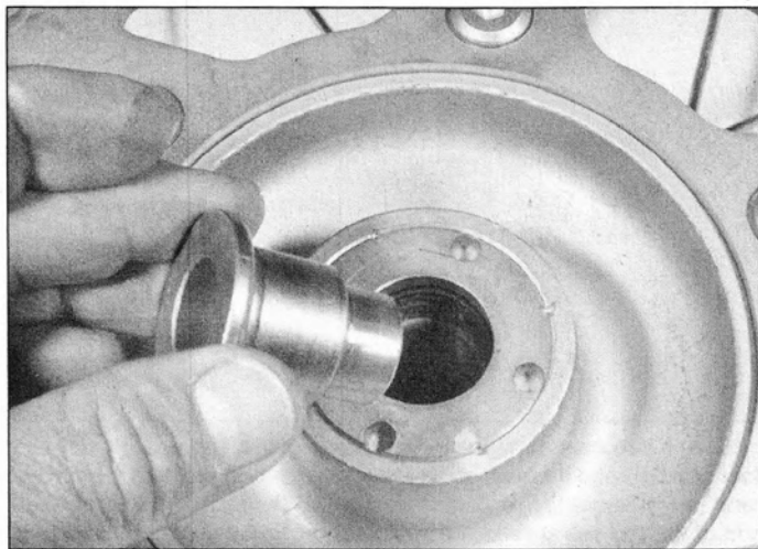
13.27 Turn the wheel over and remove the collar from the sprocket side
