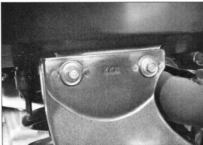
7.3 Remove two bolts to detach the inner fender
