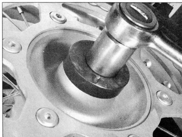
13.28c Turn the shaft with a socket or wrench to unscrew the retainer from the hub
