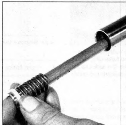
4.2k . . . and remove the damper rod from the inner fork tube
