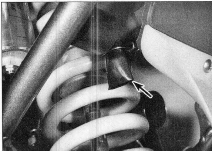
12.8a Open the drain tube (arrow) to release accumulated oil and water; if it's clogged, remove it for cleaning . . .
