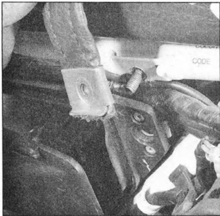
2.2 On XR250L models, remove the seat strap nut on each side and pull the strap off the studs . . .
