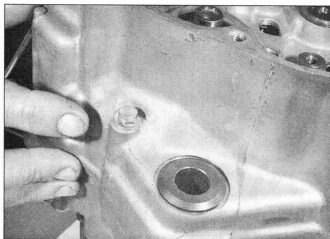
23.11b . . . on XR400R models, remove one bolt from the right side of the case near the rear of the engine . . .
