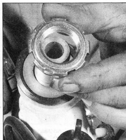
5.7a Remove the bearing adjusting nut ...
