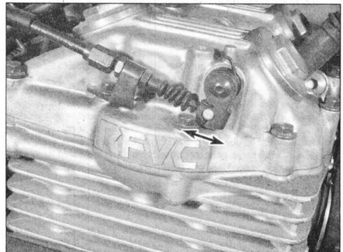
18.2 XR250L decompressor freeplay is measured at the lever
