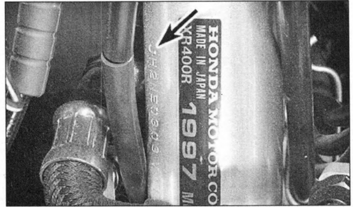
The frame serial number is located at the front of the frame
