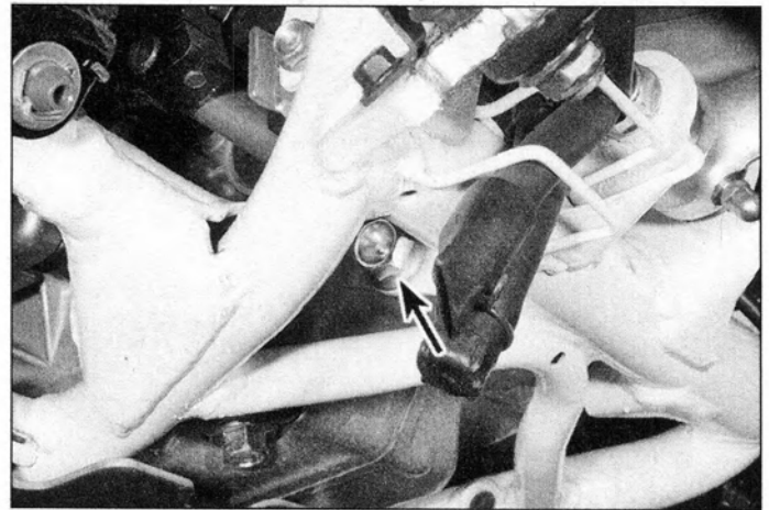
5.14e ... then remove the through-bolt from the lower rear of the engine
