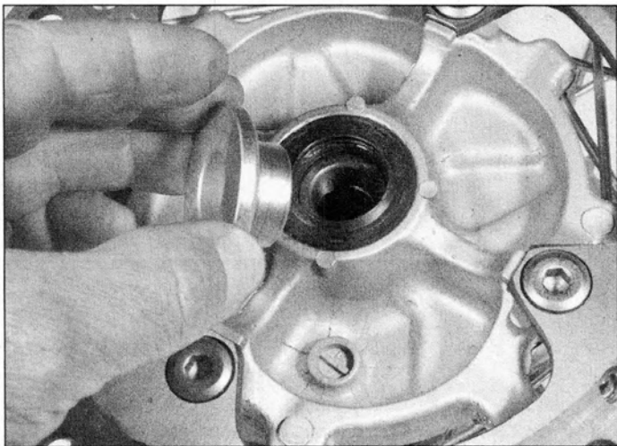
13.26 Remove the collar from the disc side of the wheel
