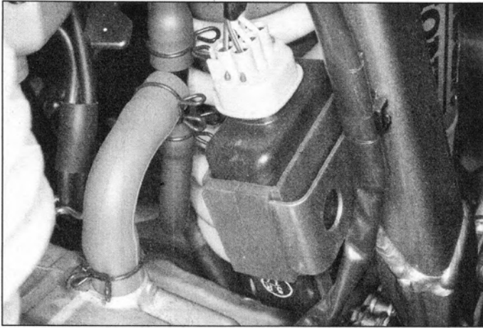
22.4 The XR400R ICM is mounted on the frame
