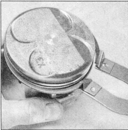
14.6 Remove the piston rings with a ring removal and installation tool
