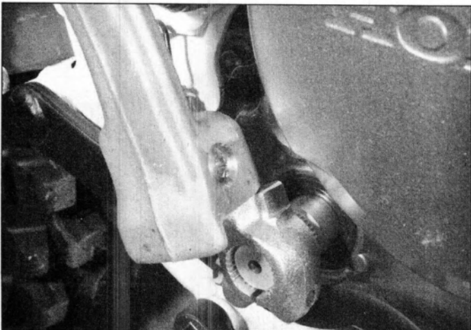
21.2 The pedal is secured to the lever by a screw
