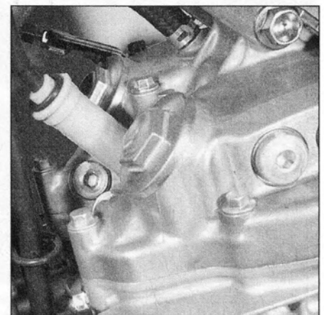
15.1 Twist the spark plug cap back and forth to free it, then pull it off the plug
