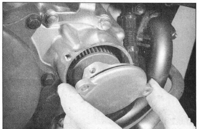
11.6a Remove the Allen bolts (some models use only two), then pull off the oil filter cover and O-ring ...
