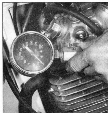
16.5 A compression gauge with a threaded fitting for the spark plug hole is preferred over the type that requires hand pressure to maintain the seal
