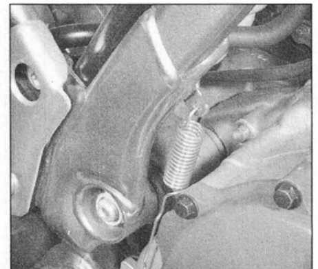
8.5 The brake pedal spring on later XR250R and all XR400R models is hooked to the frame
