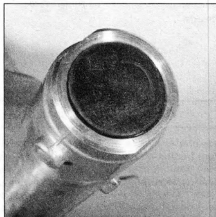
3.3c If you're planning to disassemble a cartridge fork, pry the plug out of the bottom of the fork . . .
