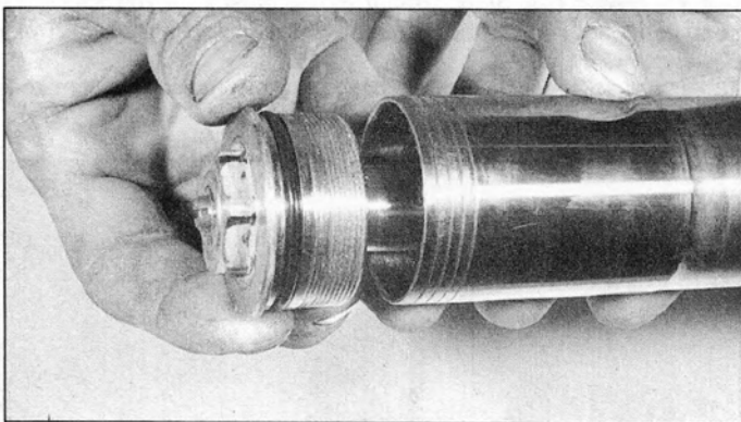
4.19 Unscrew the cap bolt from the fork (XR400R shown)
