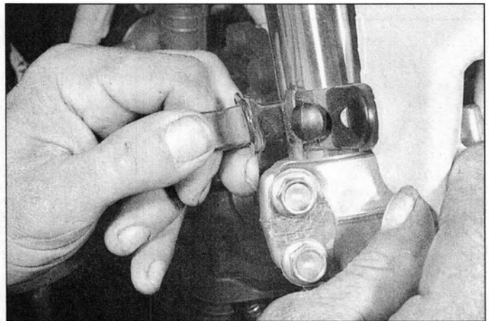
6.6a The 1986 through 1995 XR250R and XR400R headlight housing is secured by four rubber retainers
