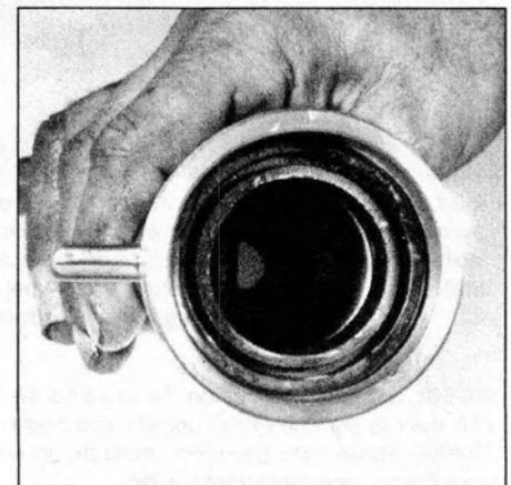
4.2l Pry the oil seal out of its bore; be careful not to scratch the seal's seating area in the fork tube
