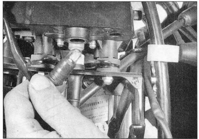
6.22 Pull the bulb socket out of the cluster, then pull the bulb out of the socket
