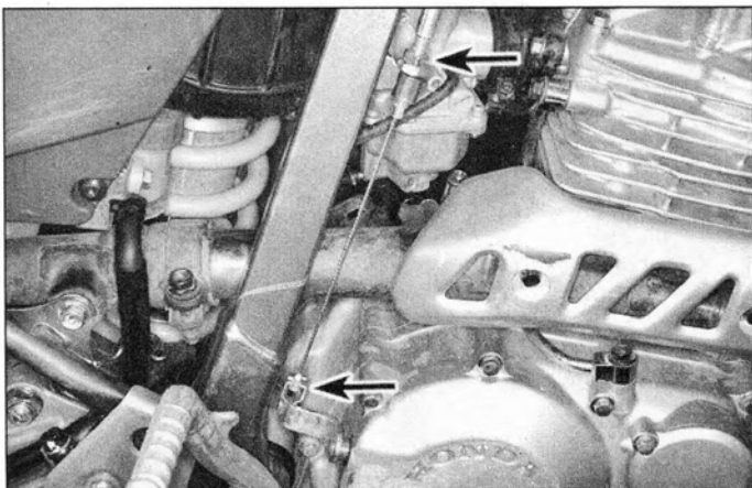
16.2 The XR250L and XR250R clutch cable runs down the back of the engine; loosen the locknut and adjusting nut (upper arrow) and slip the cable out of the bracket, then slip it out of the lifter lever (lower arrow)
